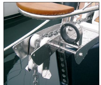
Bow fittings on some boats can be integrated with the bow anchor fitting.
